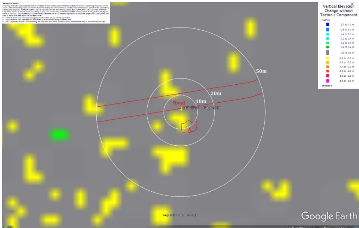
Figure 36: Ground surface subsidence without tectonic component for Dec 2011 Earthquake according to the LiDAR DEM.
